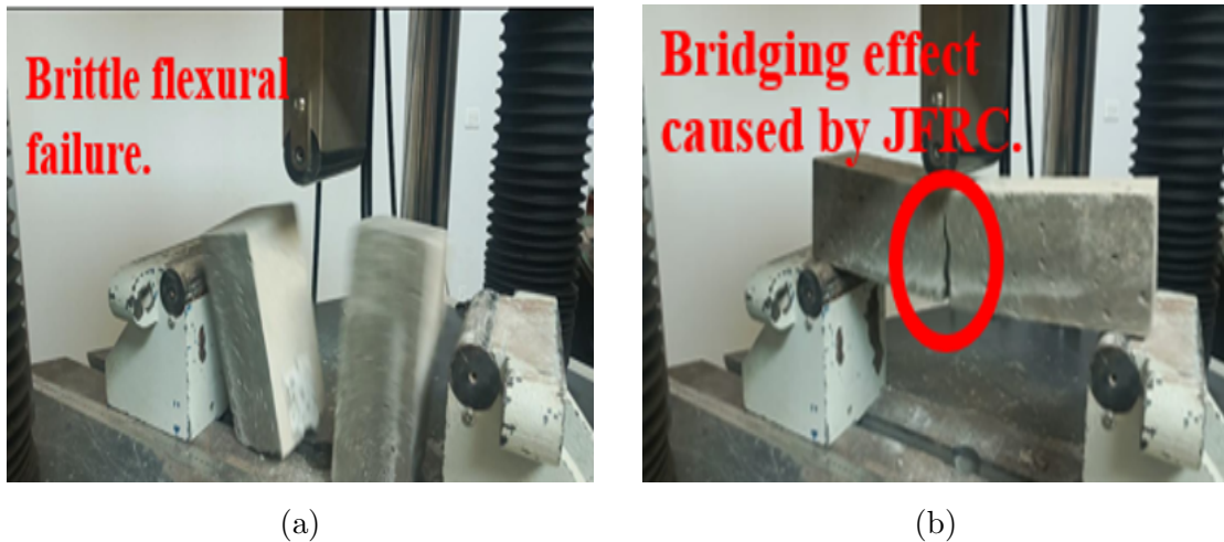
FIGURE 4.6: Crack patterns of (a) PCC and (b) JFRC specimens under flexural loading conditions
