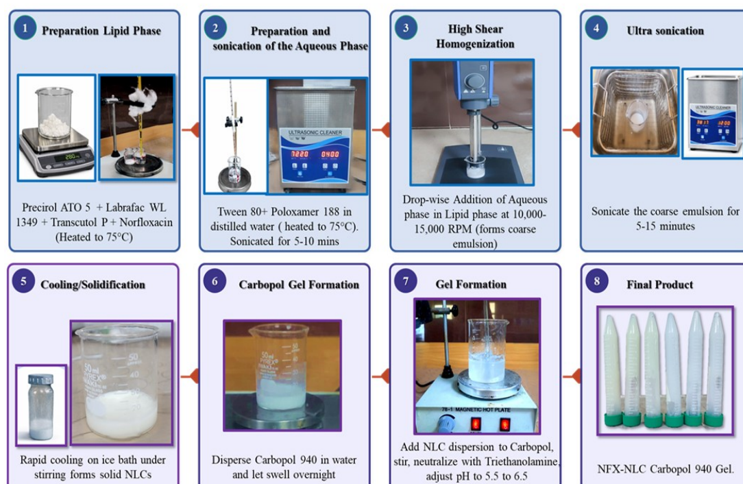
FIGURE 3.2: Schematic diagram of the preparation of NFX loaded NLC based Carbopol Gel
