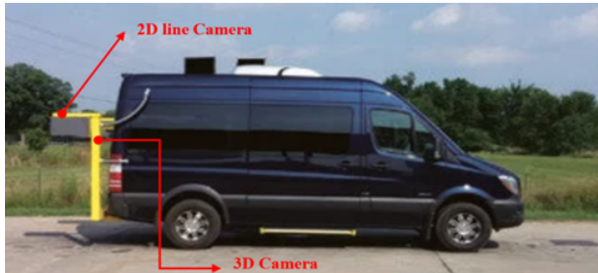
FIGURE 2.2: PavVision3D Ultra System equipment with 2D and 3D camera sensors [33]
