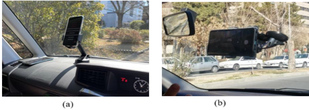
FIGURE 2.13: Mobile-Based Data Collection Setup for Pavement Distress Detection (a) Dash-mounted mobile device [99]. (b) Smartphone mounted on front windscreen [100]
