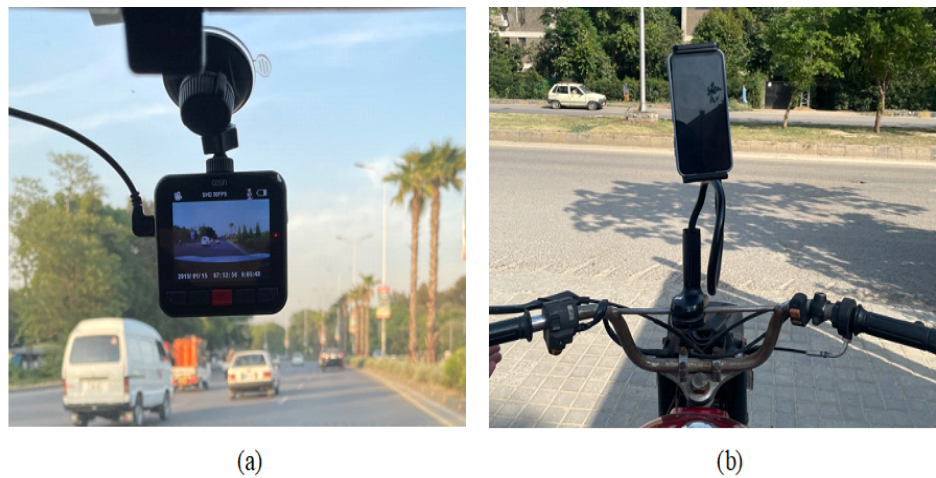
FIGURE 3.3: Mobile-based system for data collection (a) DVR camera mounted on car windshield. (b) Gooseneck Mobile holder assembly mounted on motorcycle handlebar.
