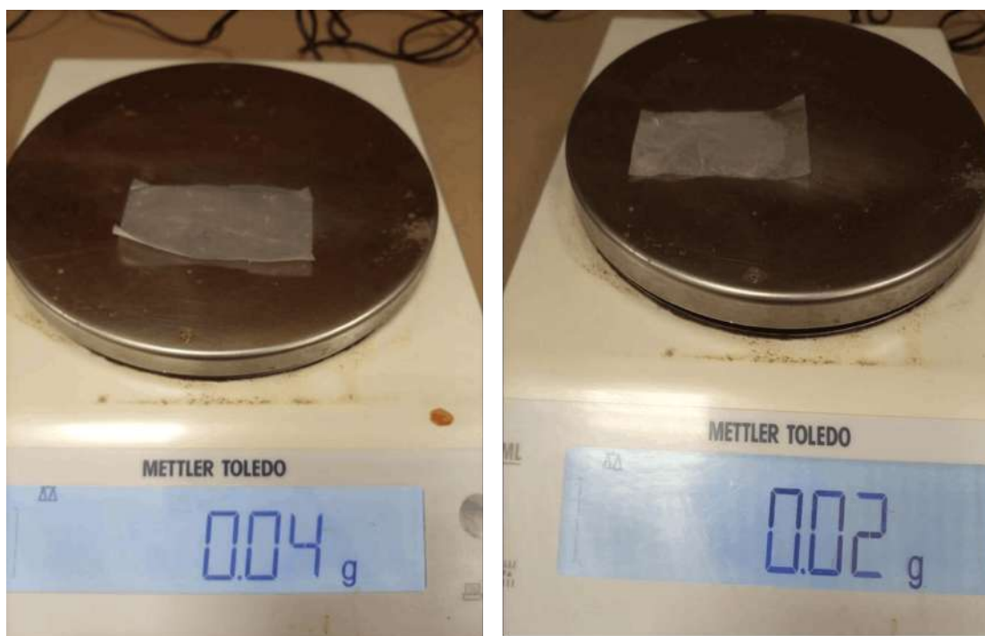
FIGURE 4.9: Weight measurement of polyethylene sample before and after degradation using analytical balance.
