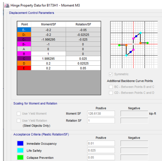
FIGURE 3.4: Defination of M3 plastic Hinge
