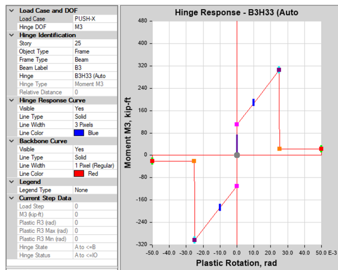
FIGURE 4.4: Beams 24 hinge not even reaching IO level
