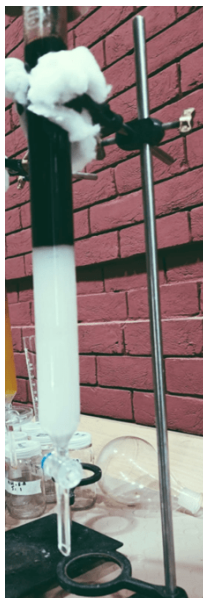
FIGURE 4.5: Column filled with the stationary phase and eluent used for Column Chromatography
