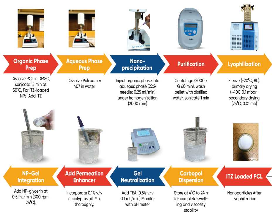
FIGURE 3.1: Schematic Diagram of the Nanoprecipitation Method for ITZ-PCL Nanoparticle Preparation
