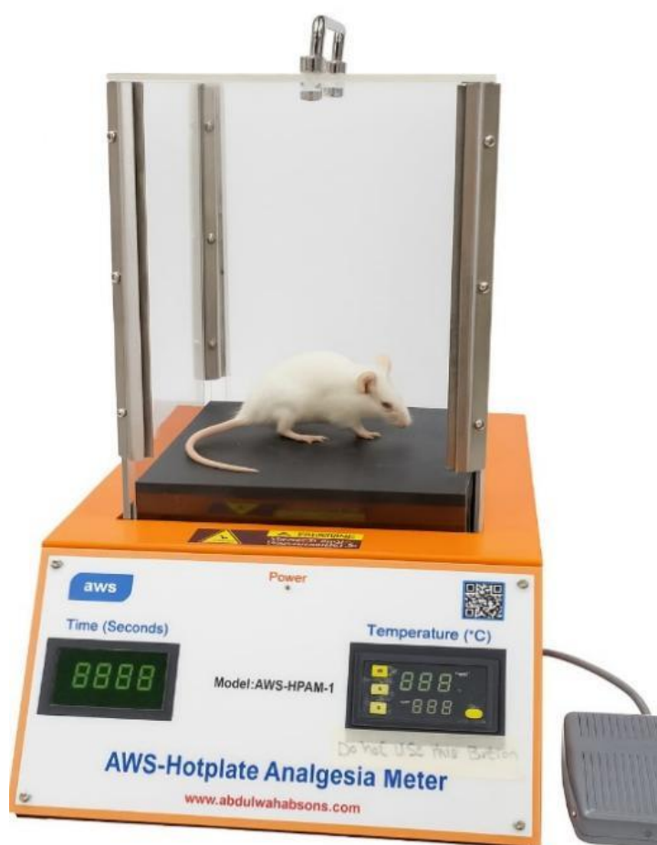
FIGURE 3.8: Hot plate apparatus used for evaluating thermal hyperalgesia in rodents
