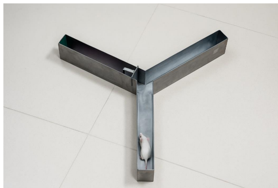
FIGURE 3.8: Y-maze apparatus for spatial learning memory assessment in mice.
