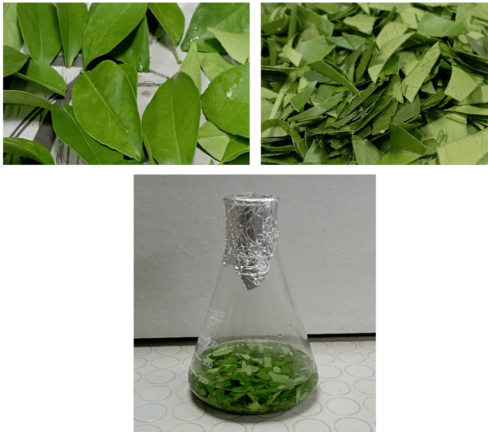
FIGURE 3.3: Citrus limetta leaves washed, dried and chopped. Then added into distilled water.
