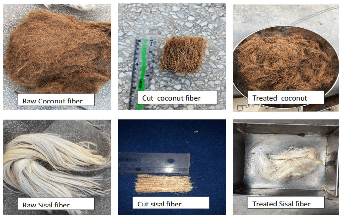
FIGURE 3.1: Images of Coconut Fibers (Raw, Treated, Cut Lengths Used) and Sisal
