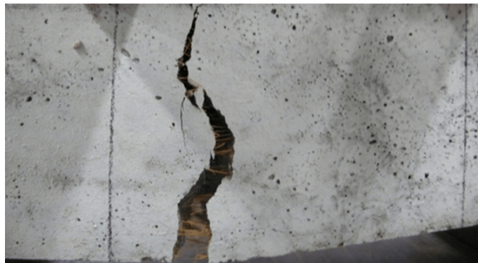
FIGURE 2.1: Natural fibres bridging crack [40].
