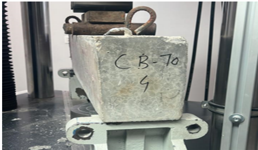
FIGURE 3.36: Beam to be loaded 70% of CB ultimate load
