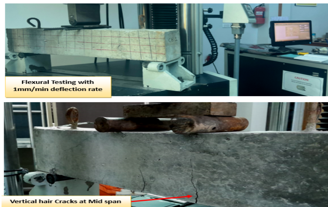
FIGURE 3.35: Flexural Testing with 1mm/min deflection rate
