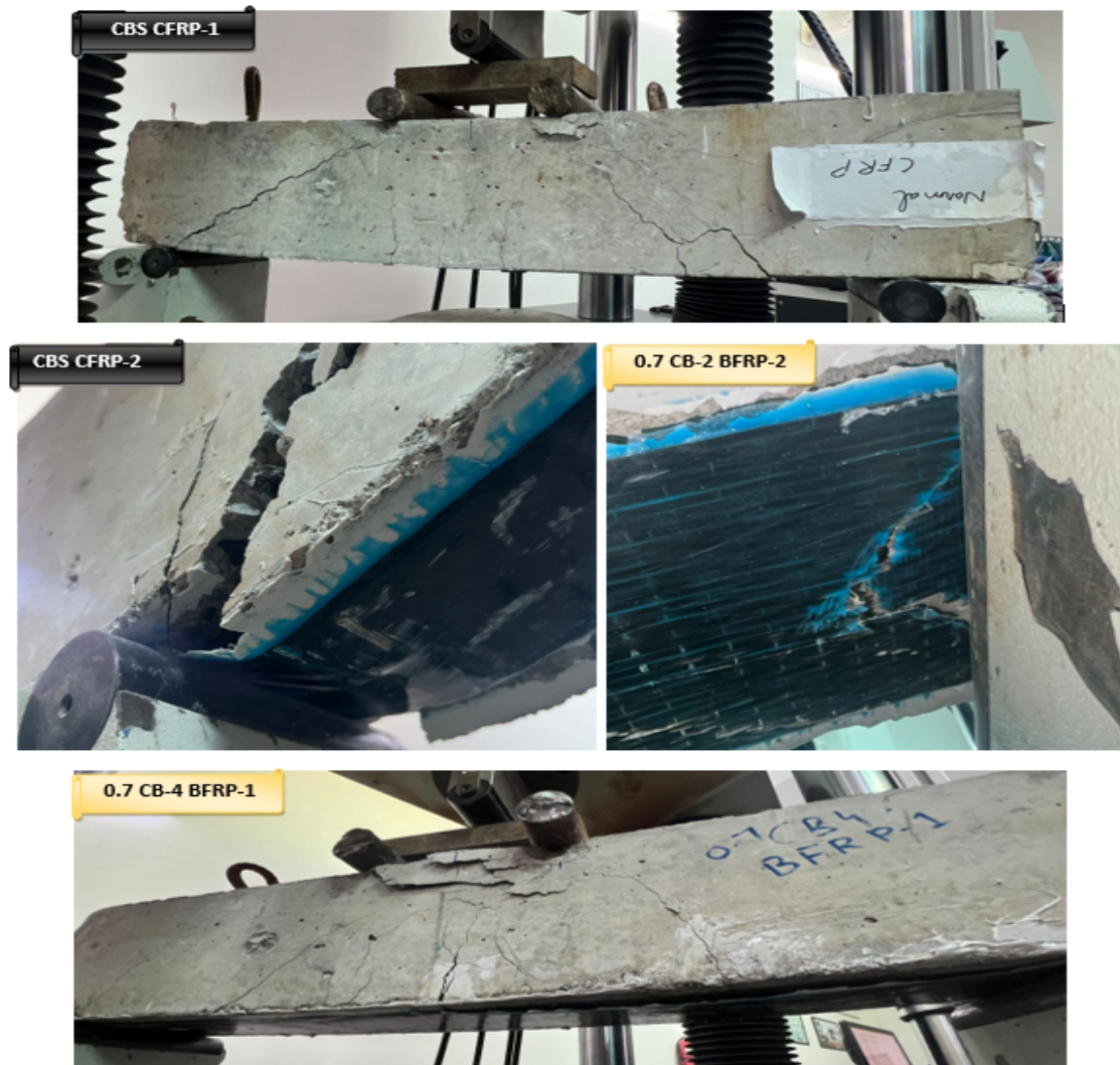
FIGURE 3.43: Flexural testing of other CFPR and BFRP beams
