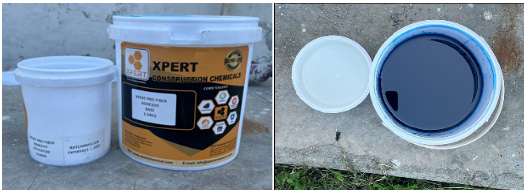
FIGURE 3.7: Adhesive in two parts and mixed with ratio of 2:1
