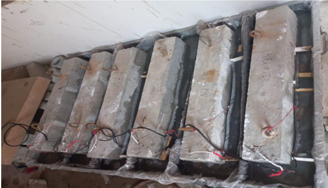
FIGURE 3.21: Physical interpretation of Schematic circuit of beams connected in series
