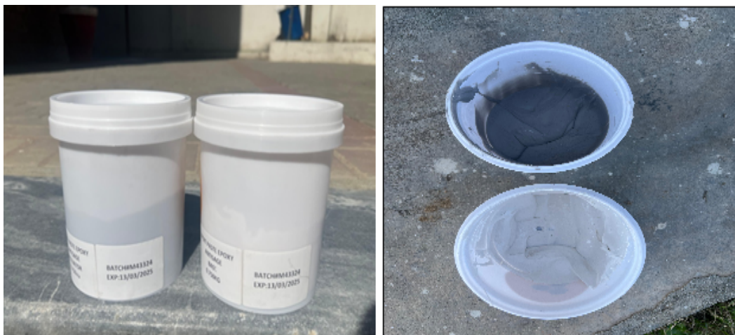
FIGURE 3.6: Base Paste Epoxy Part A and Part B, mixing ratio 1:1
