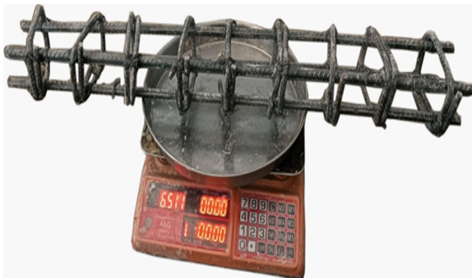
FIGURE 3.17: Total weight of beam steel skeleton before corrosion
