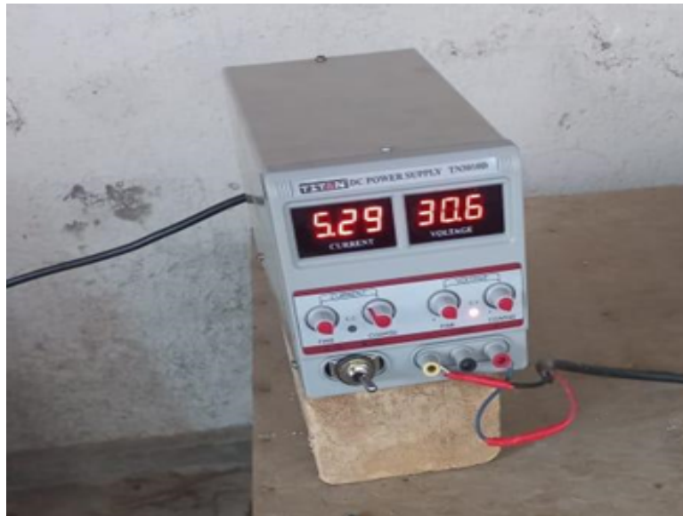
FIGURE 3.18: DC Power Supply operating above 5A current
