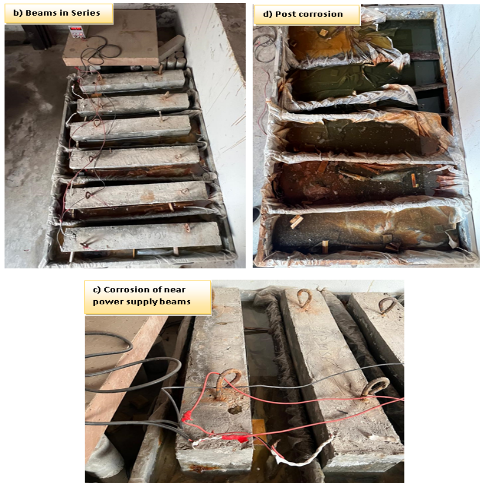
FIGURE 3.22: Beams under corrosion stage
