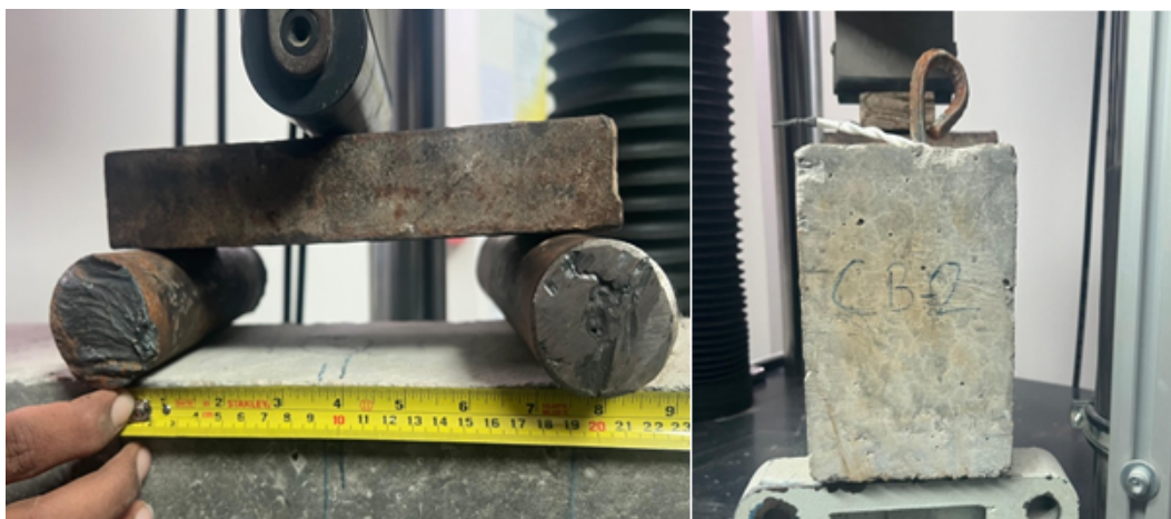
FIGURE 3.34: Rods & Wrought iron plate for four point loading
