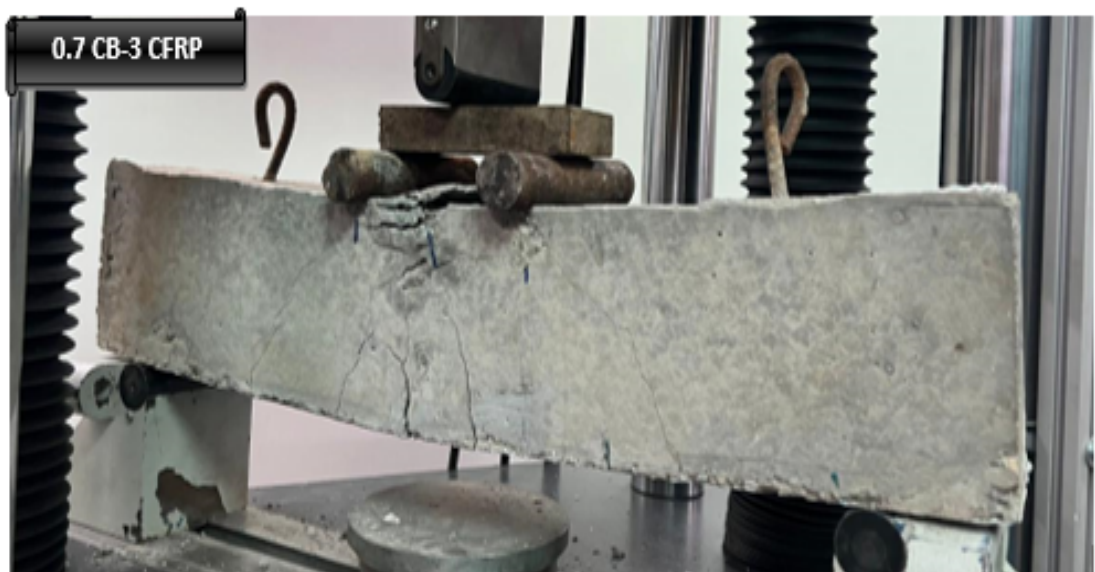
FIGURE 3.42: Flexural testing of CB-CFRP
