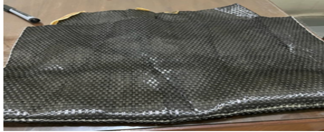
FIGURE 3.3: Carbon Fiber Reinforced Polymer (CFRP) Uni-Directional
