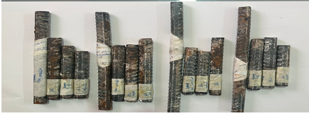
FIGURE 3.47: Cut pieces from flexural bars
