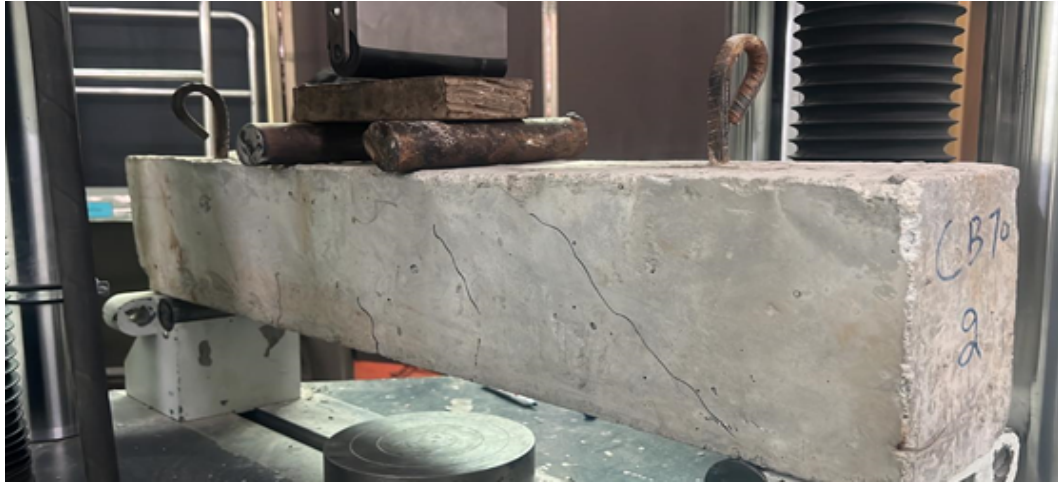
FIGURE 3.38: Diagonal cracks originating from tension zone
