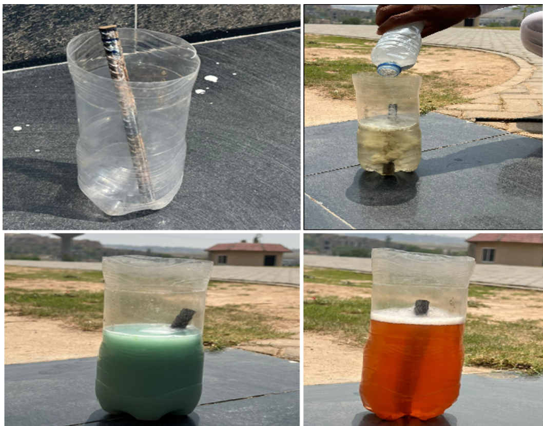
FIGURE 3.49: Procedure to remove rust from corroded steel pieces
