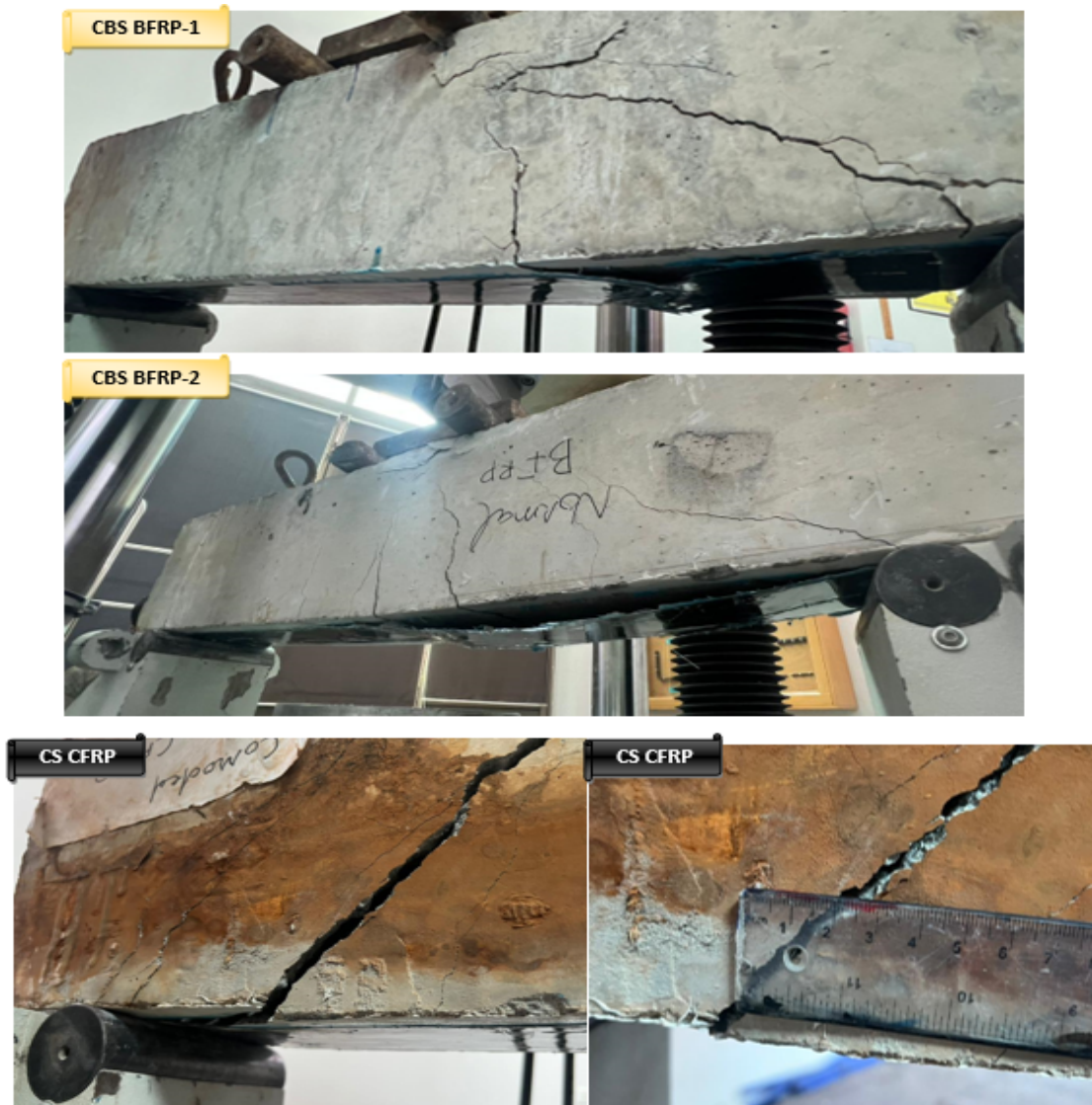
FIGURE 3.41: Flexural testing of CBS BFRP and CS CFRP
