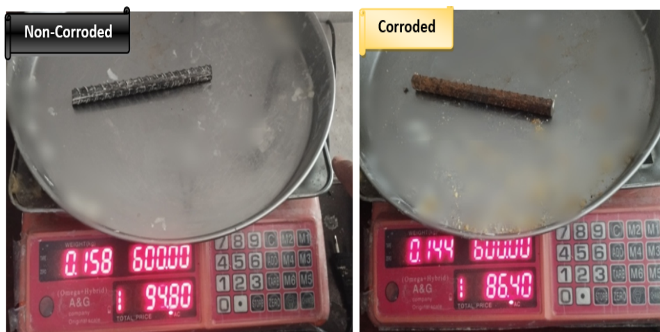
FIGURE 3.50: Comparison of weights from flexural bars away from cathode and far corner
