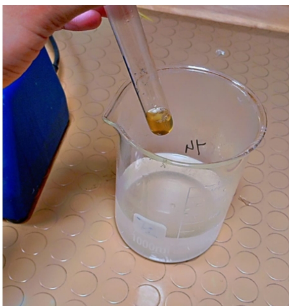
FIGURE 3.4: Checking the solubility of Hibiscus rosa sinensis mucilage by dissolving in different solvents
