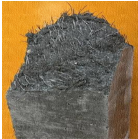
FIGURE 2.7: Fiber Reinforced Concrete for rigid pavement [11].
