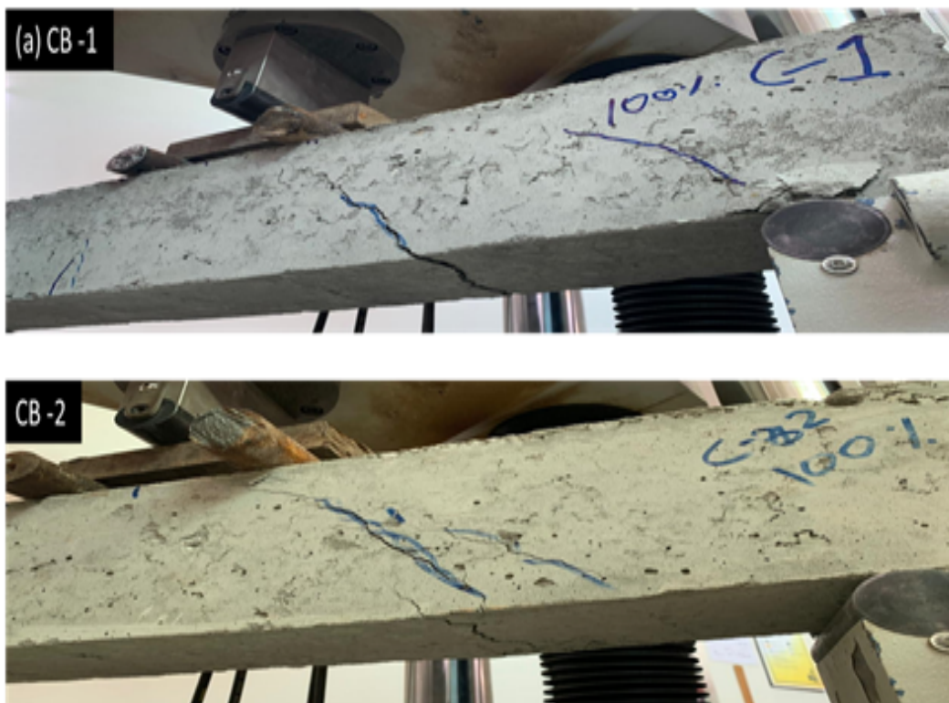
FIGURE 4.1: Behaviour beams specimen under 100% initial loading (a) CB-1 (b) CB- 2
