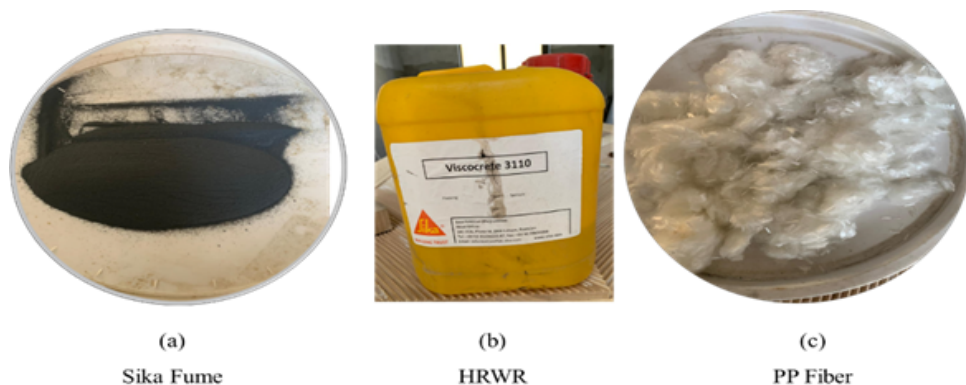
FIGURE 3.1: Raw Material used in UHPC
