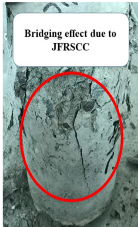
FIGURE 4.4: Bridging effect caused by JFRSC
