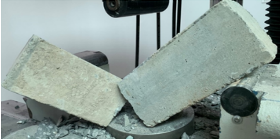
FIGURE 4.7: Beam Failure under Loading
