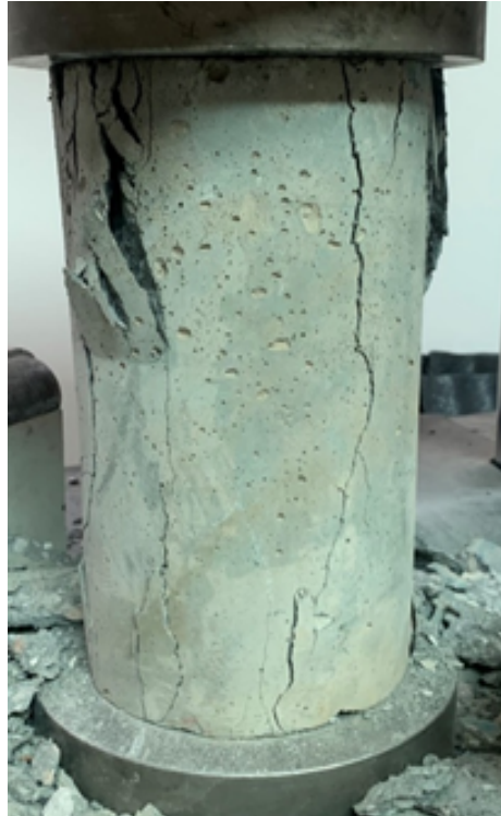
FIGURE 4.3: Spalling under compression
