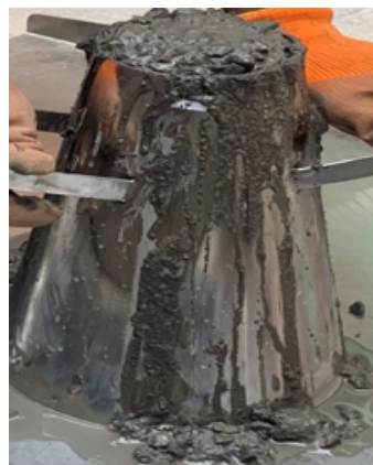
FIGURE 3.2: Flow Table Test Setup
