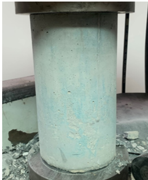
FIGURE 3.4: Compressive Strength Test Setup
