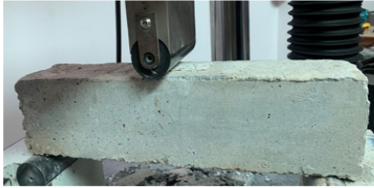
FIGURE 3.5: Flexural Strength Test Setup
