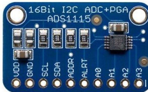
FIGURE 3.9: ADS1115, 16-bit Analog to Digital Converter
