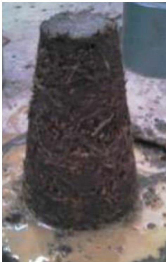
FIGURE 4.1: Measuring Value of Slump of HNS-FRCs
