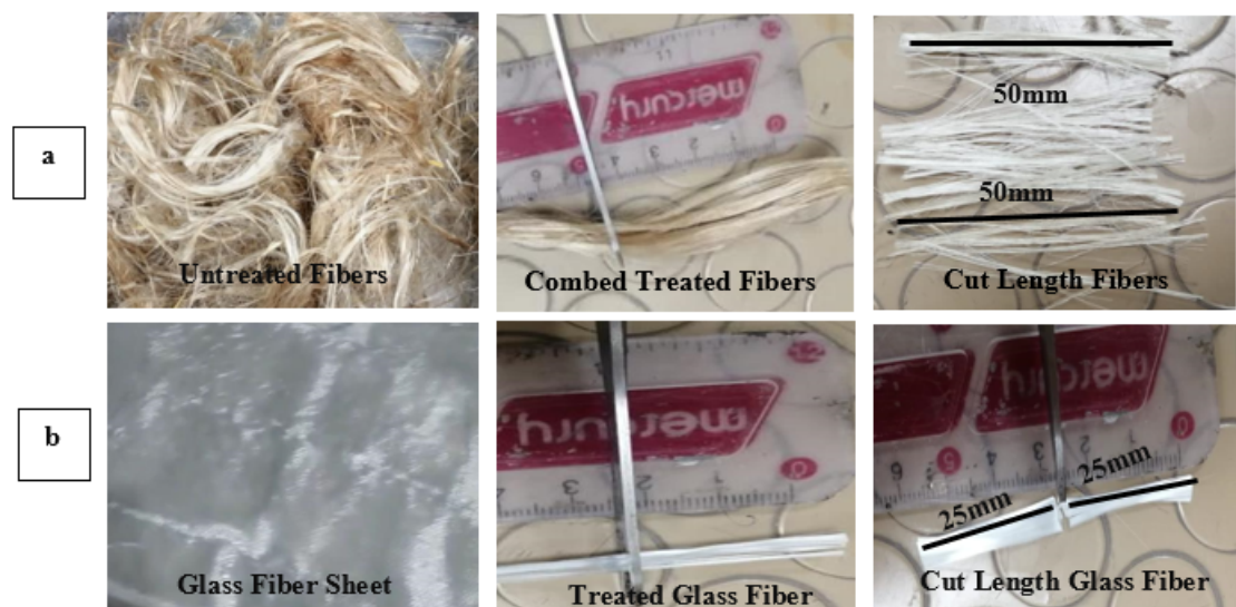
FIGURE 3.1: Considered Natural and Synthetic Fibers; a) Jute Fiber, b) Glass Fibers
