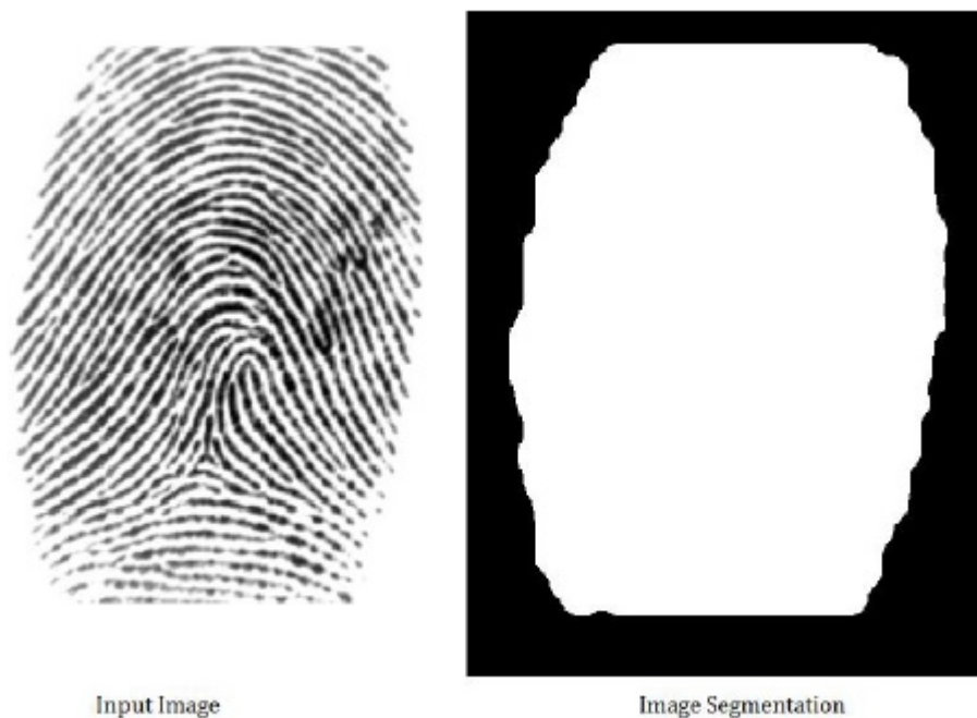
FIGURE 2.2: ROI segmentation based on Variance technique
