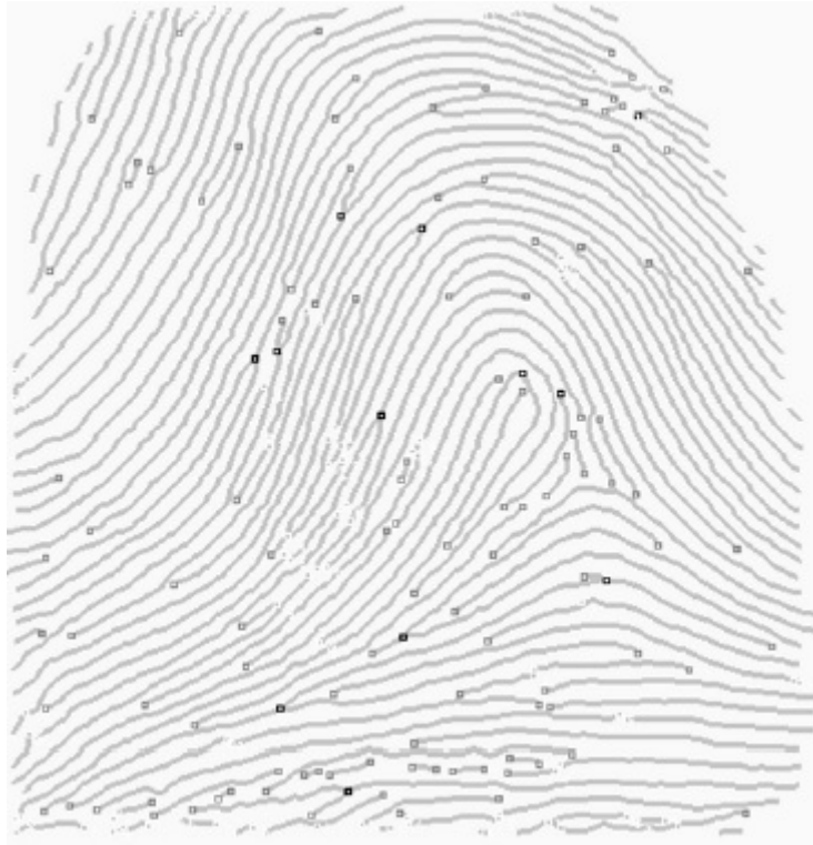
FIGURE 2.13: Result of minutiae extraction
