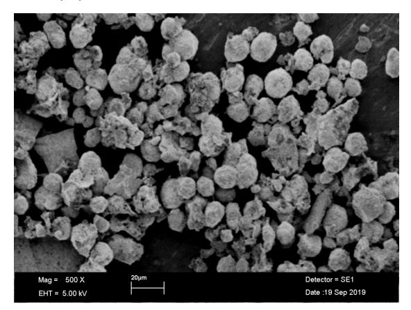
FIGURE 4.3: SEM Analysis of Synthesized Silver Nanoparticles
