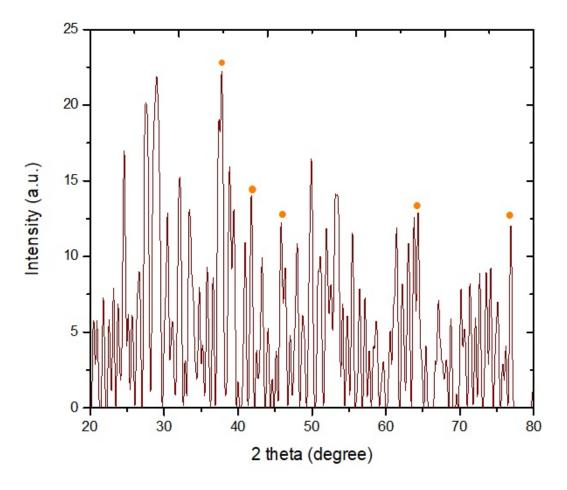
FIGURE 4.5: XRD Peak Diffractogram of Silver Nanoparticles
