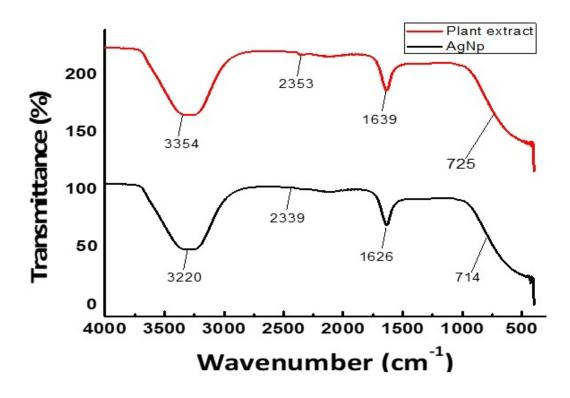
FIGURE 4.6: FTIR Spectrum of Silver Nanoparticles and Plant Extract
