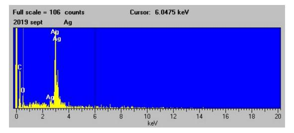
FIGURE 4.4: EDS Spectra of Synthesized Silver Nanoparticles
